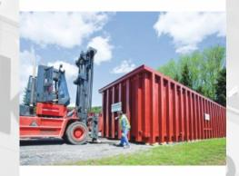
The KVK-tanks are built from panels which have a special sandwich-construction:an impact-resistant core of synthetic ceramic, coated on both sides with fibre-reinforced laminates to form an inseparable piece. The resulting exceptionally high impact strenght resists even the most severe mechanical shocks.
