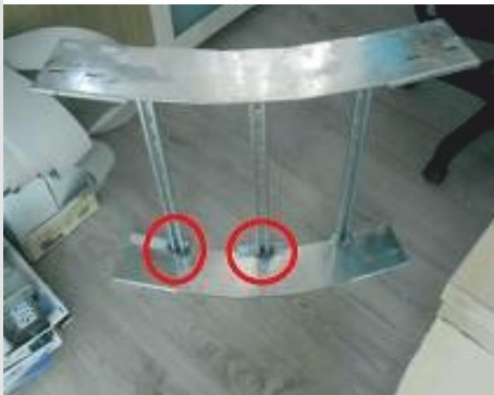
Uncoated areas in welding zone
