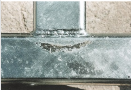
Burned oil during welding
